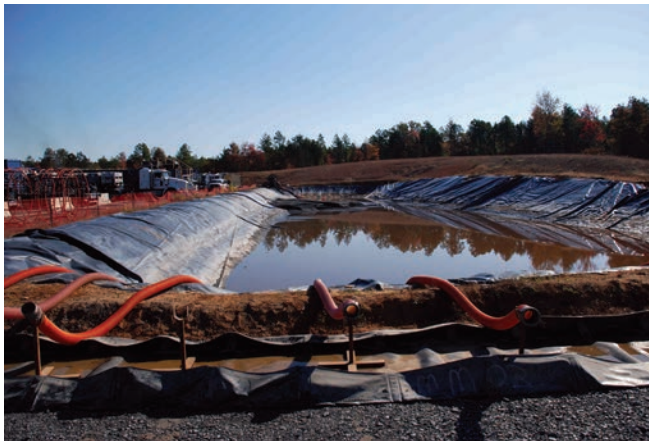
Hydraulic fracturing wastewater, including flowback and produced water, is often stored at well sites in lined pits, such as this one in the Fayetteville Shale gas play of Arkansas.
