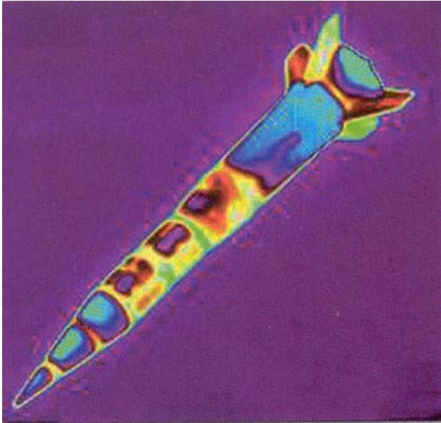
**Figure 3:** The image of the Aries target vehicle from the LEAP sensors just before intercept (US Navy photo).
