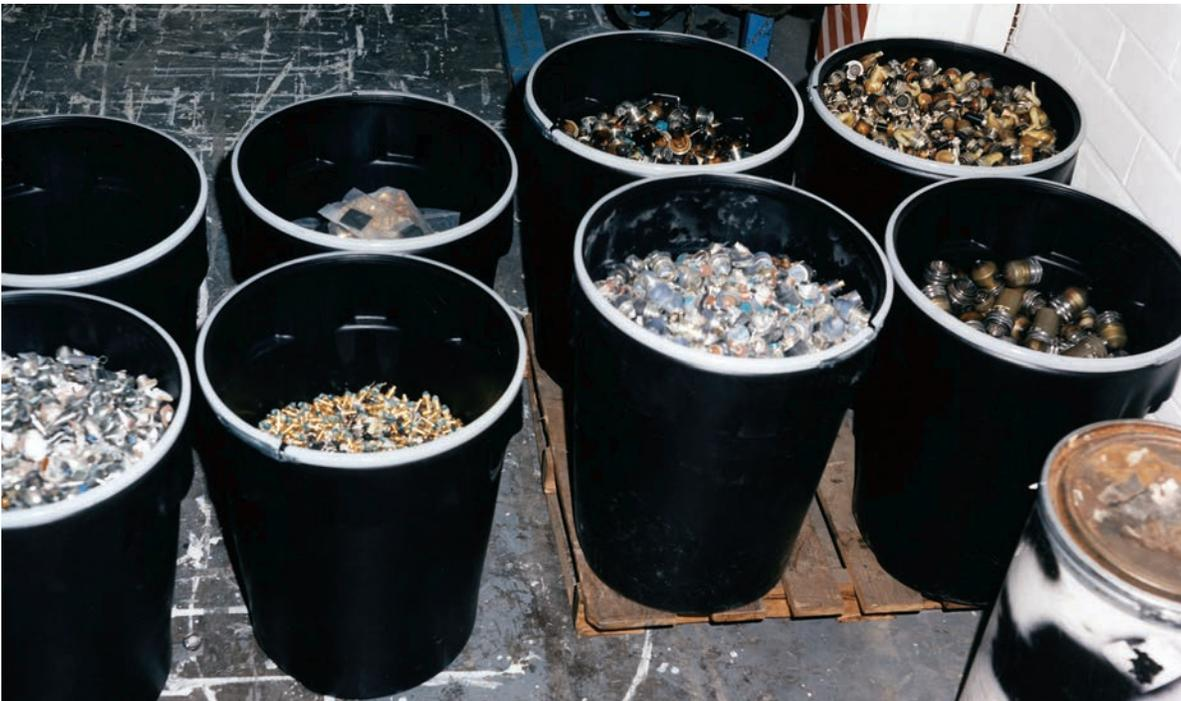
**As part of the dismantlement of warheads at the Pantex plant in Texas, copper, aluminum, silver, gold, plutonium, and non-nuclear weapons parts are separated for recycling, 1992.**
