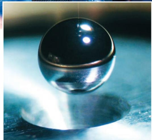
A two-millimeter-diameter capsule filled with a deuterium-tritium (DT) gas, surrounded by an 80- to 100-micrometer-thick layer of DT ice, which is the target for the lasers of the National Ignition Facility.
