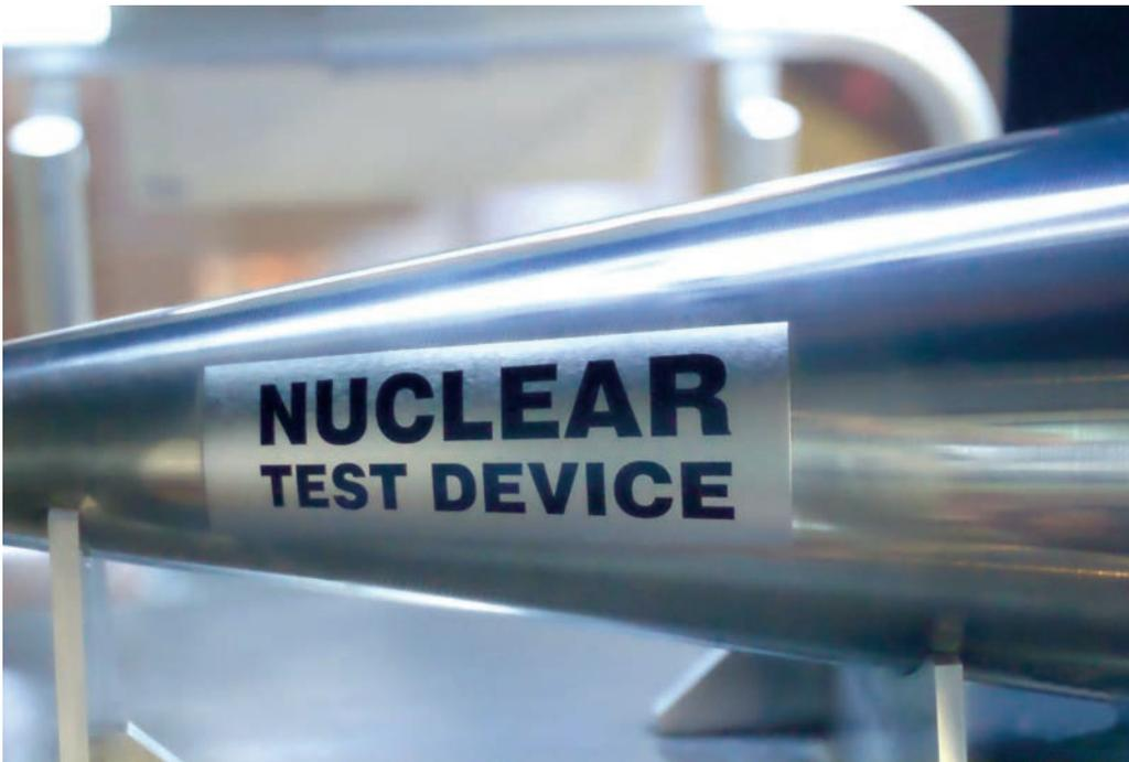
**Scale model of a nuclear weapon resting on a diagnostic rack or “jewel rack” used for weapons testing at the Nevada National Security Site. The model was built by the Los Alamos National Laboratory, Los Alamos, NM.**
