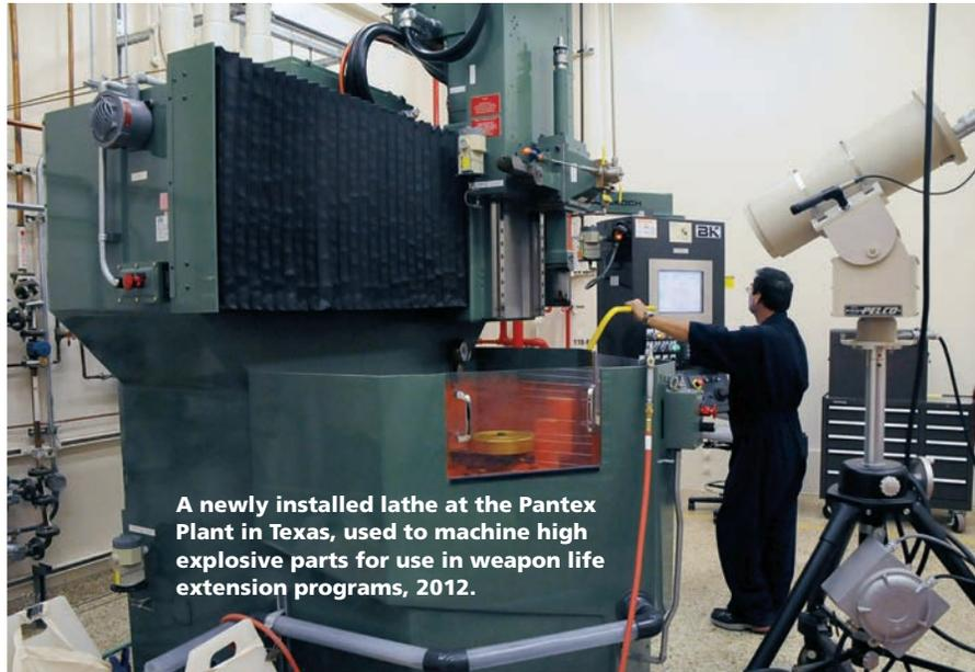
A newly installed lathe at the Pantex Plant in Texas, used to machine high explosive parts for use in weapon life extension programs, 2012.
