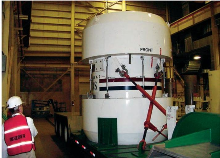
Storage cask containing transuranic waste including plutonium being put on a trailer at the Waste Isolation Pilot Plant (WIPP) in New Mexico, 2002.
