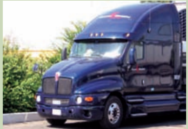
Aerodynamic-style tractor with low-profile front, aerodynamic bumper, full-height roof fairing, hidden exhaust stacks, and fuel tank side fairings. Photo courtesy of Don Anair.
