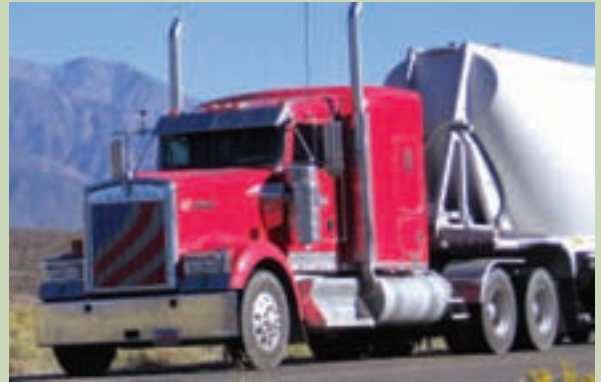
Typical classic-styled truck with long nose, flat bumper, low roof, and exposed air cleaners, exhaust stacks, and fuel tanks. Photo courtesy of Don Anair.
