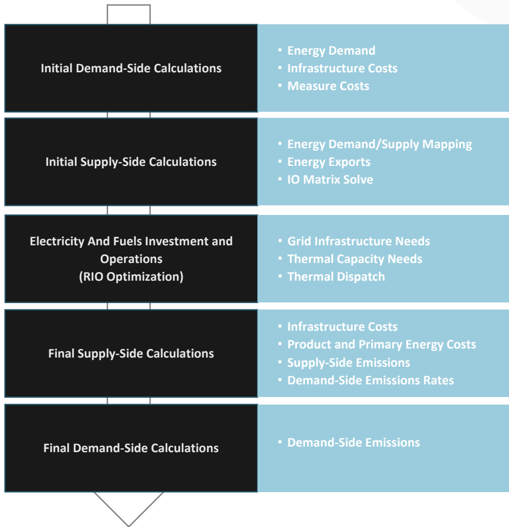
Figure 6 shows the basic calculation steps for EnergyPATHWAYS and the outputs from each step.
