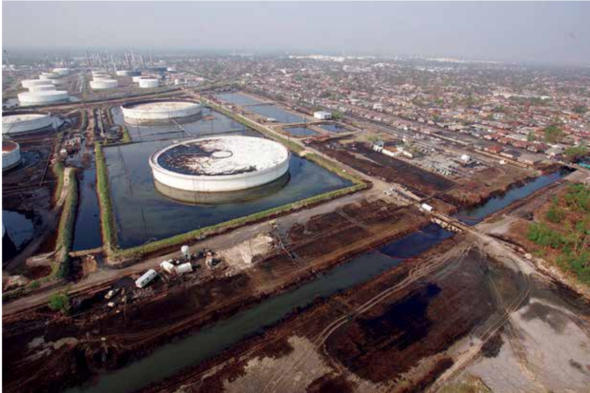
Communities like Chalmette, LA, which are located near industrial facilities, are at risk from toxic pollution in the wake of flooding. Hurricane Katrina's massive storm surge forced an oil tank at the nearby Murphy Oil Refinery from its foundation, spilling over a million gallons of crude oil into the floodwaters and nearby canals, and affecting over 1700 homes.
